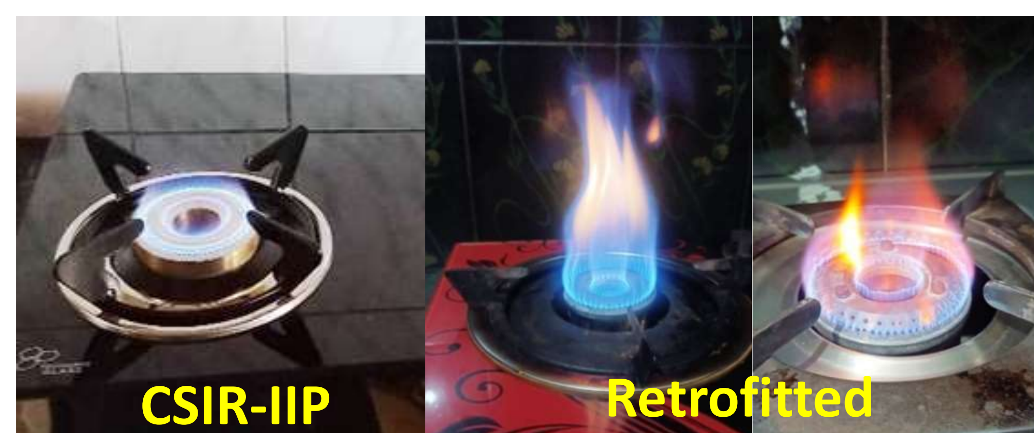
Comparison of flames of CSIR-IIP and retrofitted burners
